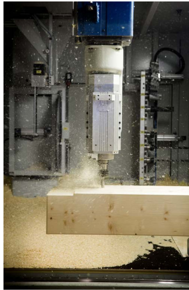
CNC machining of glulam beam.
