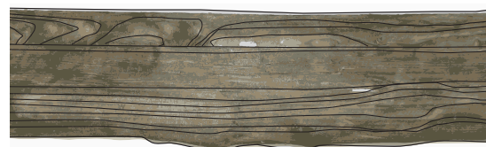
Figure 16.2 Glulam beam without significant singularities after a fire
